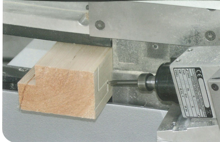
Incisore anti-scheggia Scoring unit with anti-splintering device Antisplitter-Vorfräser Incisor antiestillas Inciseur anti-éclats
