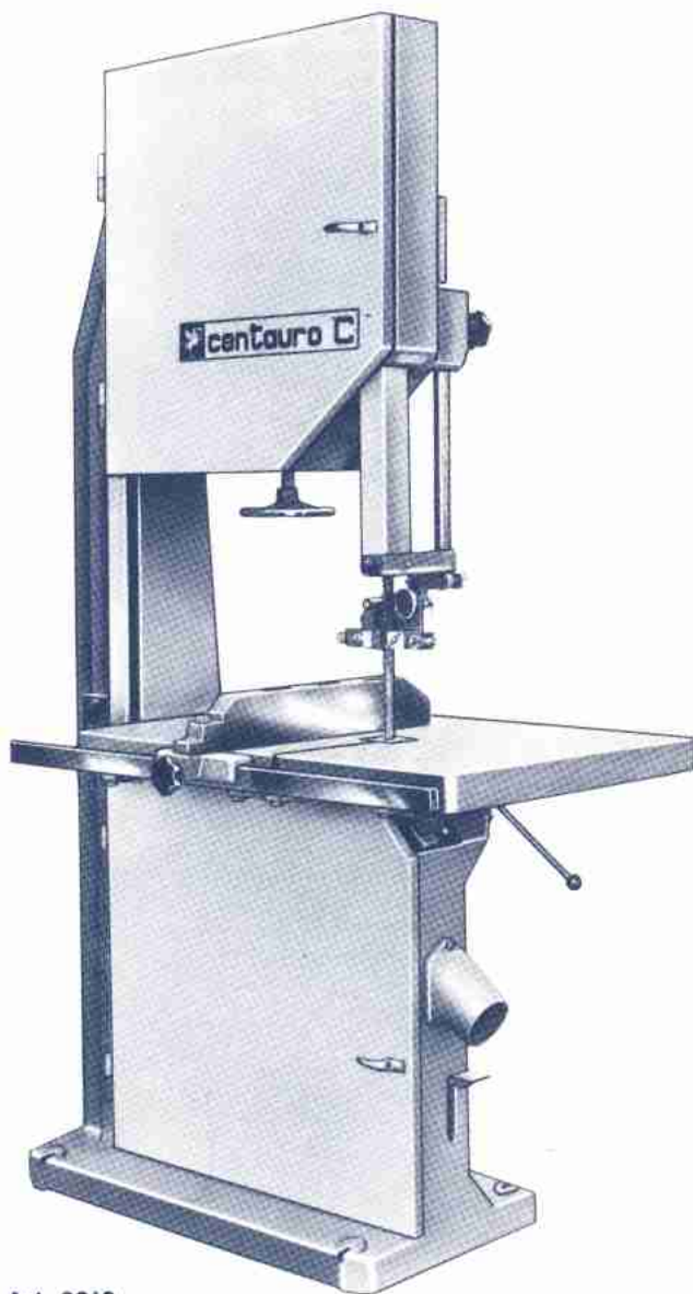
Art. 2219 Band saw classic - Mod. "CL 600" - "CL 700" - "CL 800" Cast-iron table wheels full
