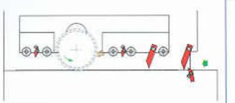
TOP ROLLERS GROUP raised automatically, with 5 independent hold-down rolls and a long wooden shoe placed between the blades. The splinterproof system consists of steel fingers distributed on 4 top rows (two of which acting as splinterproof and the other two as anti-kickback) and one bottom row.
