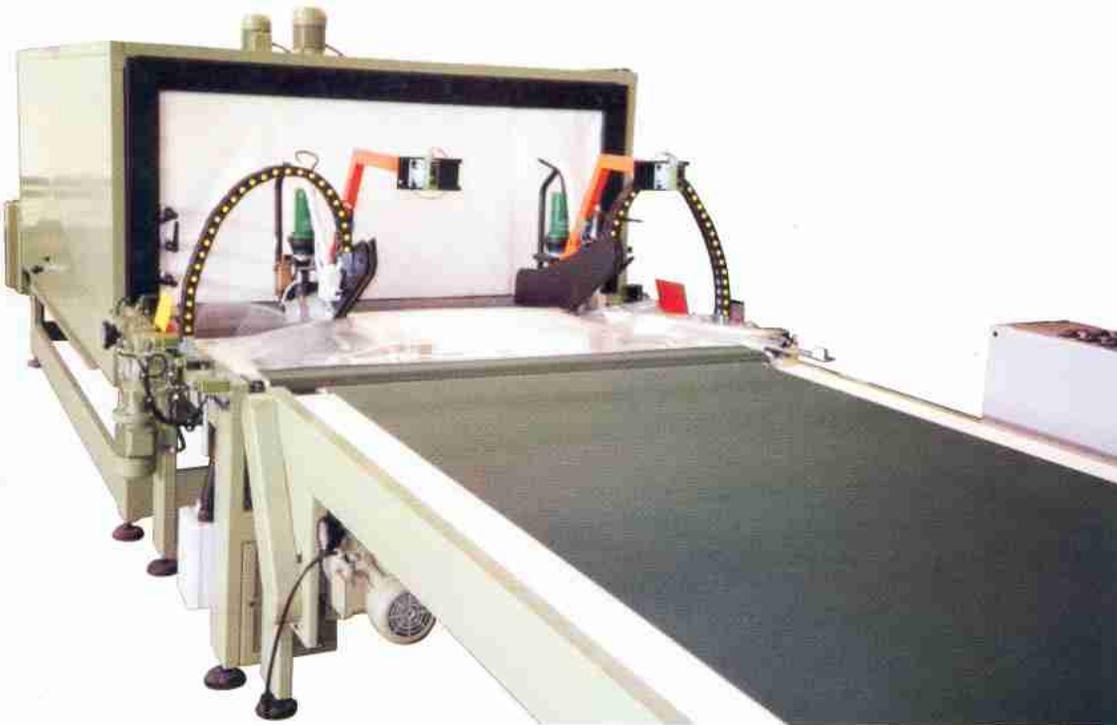
■ Side welding station to be installed in-line with a shrink wrapping line mod. STAR. Sirio is particularly suitable for flat pack furniture or low products. The cutting discs and the "Leister" blowers ensure same sealing quality as a STAR even on the sides of the product; the independent operating units, then, allow for processing a flow of items with different sizes without manual adjustment. Being a separate module, can be retrofitted in a shrinkwrapping line later on.
