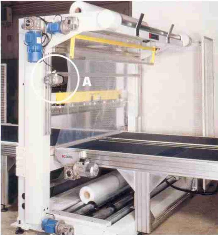
■ The wrapping station is equipped with an upper and a lower film roll, both motordriven. On request it is possible to mount up to three couples of independently motordriven foil rolls, as well as bubble wrap film rolls.
