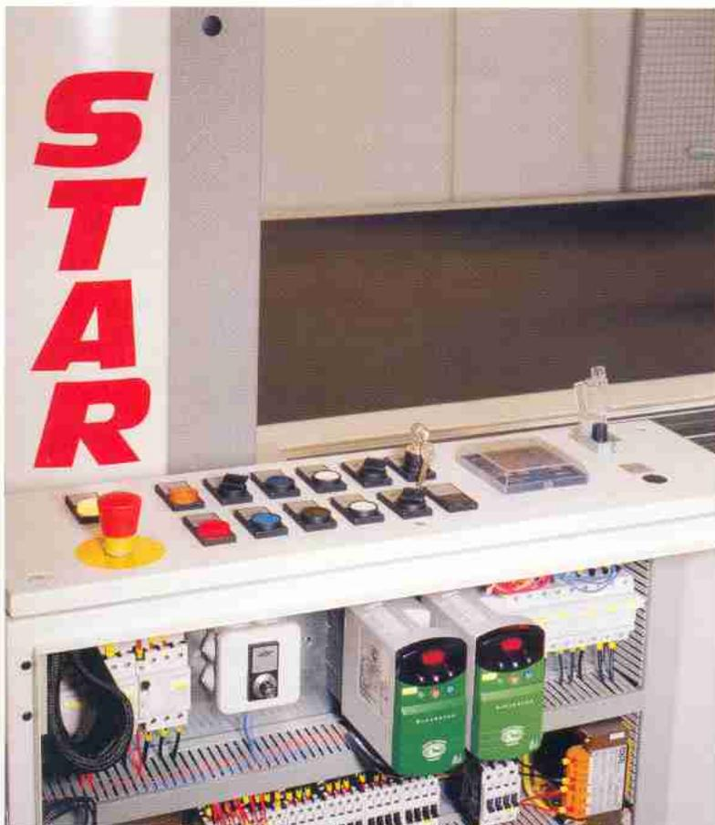
■ All the conveying sections of the machine, both in the wrapping station and in the shrink tunnel, are managed by inverters, in order to change the speeds in a flexible and independent way.
