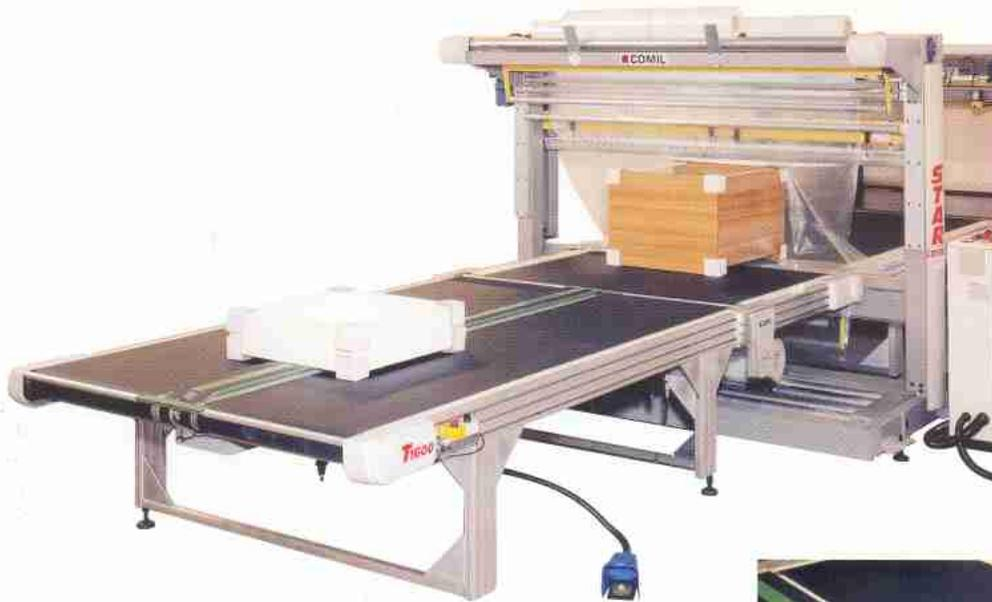
■ The conveyor belts are sized in order to cover the widest range of requirements; moreover they are independently motordriven, in order to avoid any conveying problem even with heavy items and to allow for a flexible management of the different speeds.
