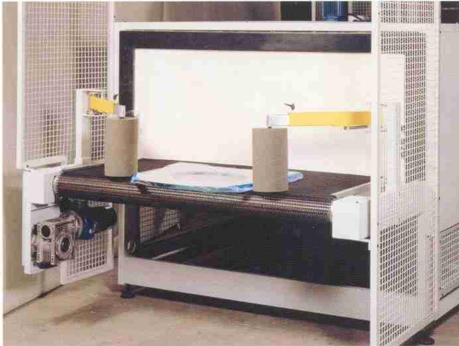
■ The conveying system in the shrink tunnel is by means of a completely teflon coated net, in order to ensure an uniform bearing surface and to avoid scratching the film during the shrink process. Moreover, being a complete revolving net, dragging chains are avoided, therefore reducing tearing and maintenance needed.
