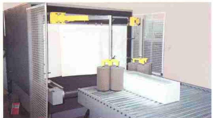
■ At the outfeed end, the shrink tunnel is equipped with a couple of side film pressing rollers, pressing the side excess of film against the product, in order to obtain a better package quality. On request it is possible to have a motor driven version, when the dimensions of the items vary remarkably.
