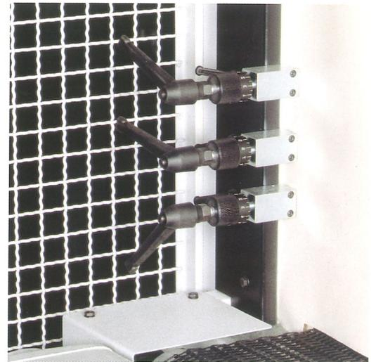
At the tunnel infeed 3 couples of knobs are located in order to modify the air flow in the shrink oven, according to the kind of items to process and the shrinking required.
