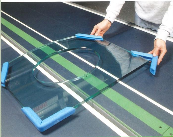
On request it is possible to equip the wrapping unit with a range of conveyors with raising middle bar with motordriven small belts. This option is particularly useful for making the package preparation easier without stopping the belt and slowing down the flow. Moreover, the additional belt section allows for a complete 3 meters long working area without interfering with the safety grids.
