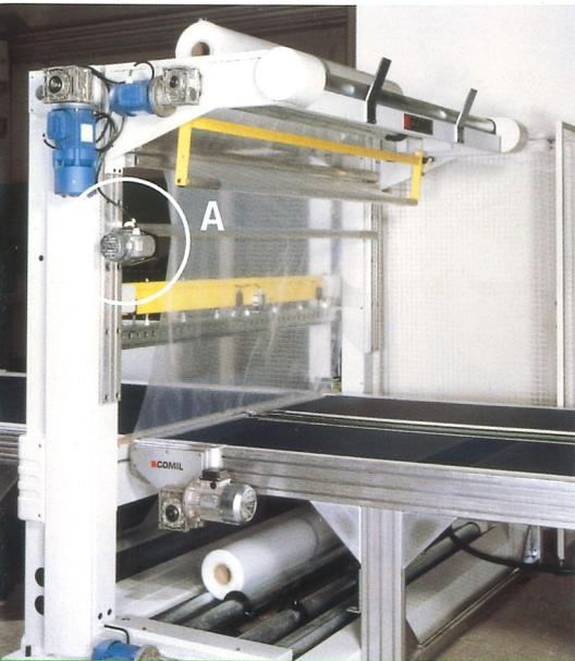
The wrapping station is equipped with an upper and a lower film roll, both motordriven. On request it is possible to mount up to three couples of independently motordriven foil rolls, as well as bubble wrap film rolls.
