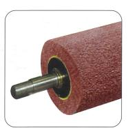
The Scotch-brite™ units are utilized to improve the sanding level of finish and to clean the lacquer surfaces. The scotch-brite brush has a structure of non-woven synthetic fibres impregnated with abrasive grain of aluminium oxide or silicon carbide, the rollers are available in variable grit (80÷1000) and various density.
