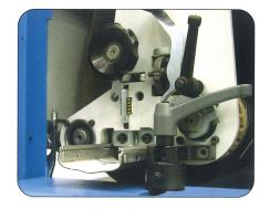
Pneumatic pad unit with electronic control of time entry of contact element. Complete with aluminium profiles for quick change of felt and graphite cloth . (CK)
