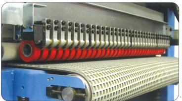
Vacuum plant with optional electro-ventilator. It is required to obtain a tighter hold of work-pieces on the feed belt, if compared with the pull obtained by connecting with the dust plant (standard feature), when the air speed/volume are too weak.
