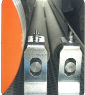
Double rollers pressure unit with micrometric adjustment positioned in-front and rear of each working unit
