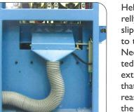
Help holding securelly small and/or slippery work-pieces to the feed belt. Need to be connected to the main dust extraction system that must have a reasonable speed of the air flood.
