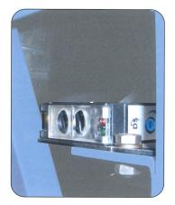
Sanding belt oscillation by special photocell with double eye.
