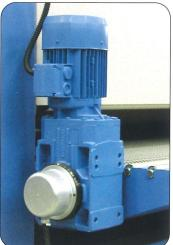
Feed speed variable in continuous from 3 to 15 m/min controlled by inverter
