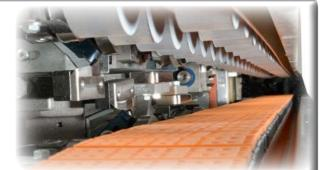
■ The presure bar, made from two rows of idle rubber rollers, is adjustable by a handwheel complete with a mechanical numerical indicator. The irreversible mechanism (selflocking) with conical gears, assures a precise and stable positioning.
