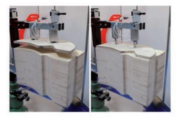
Provided with a pneumatic lock to fasten the material, it allows to overlap the panels, placing the template on top of them.
