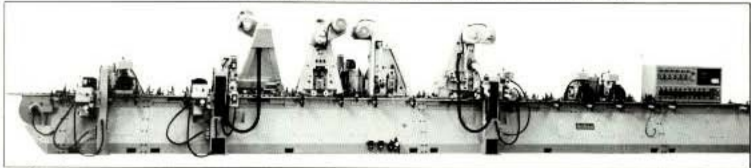
Ten Station Sander with a multiple Belt and Wheel Unit Configuration
