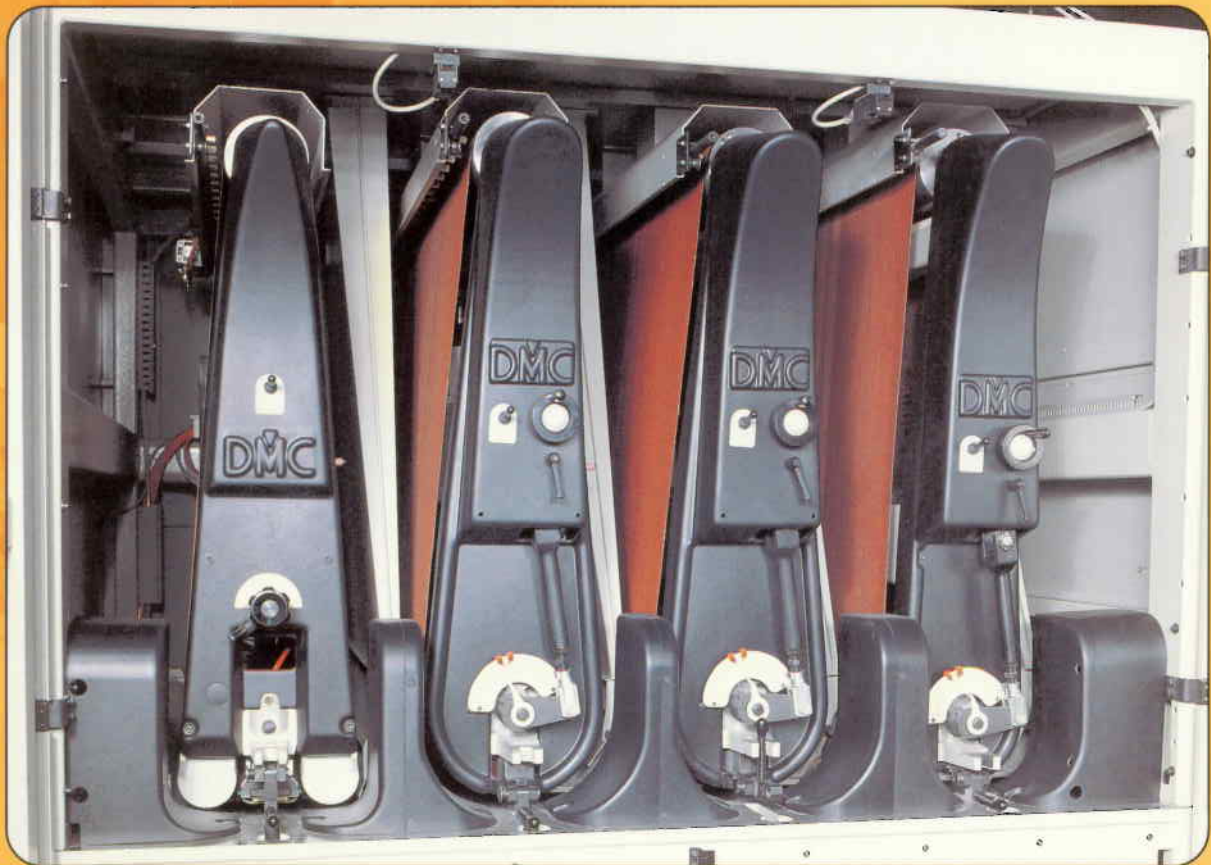
M4 250 mm Roller - 250 mm Roller - 320 mm Roller - EPICS Pad Walze 250 mm - Walze 250 mm - Walze 320 mm - Schleifschuh EPICS
