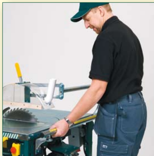
Mounting/demounting of guide bar without tools
