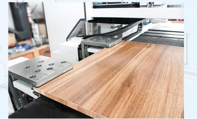
Grippers are automatically positioned to accommodate different sized workpieces
