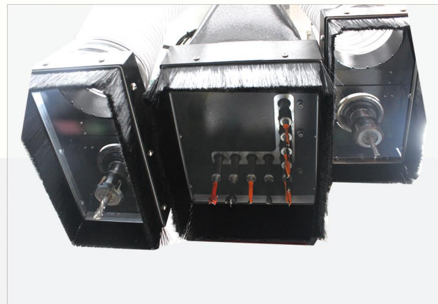
Two spindles, one for nesting, one for grooving, or have it your way—the two manual tool changing spindles work together and eliminates half the tool-changing time. 5+4 Vertical Drill Bank is standard feature.
