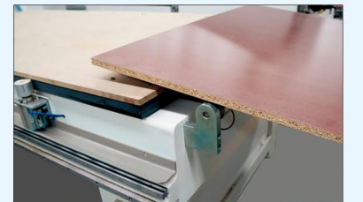
Rollers located at the front and rear end of the machine for easier loading and off-loading.
