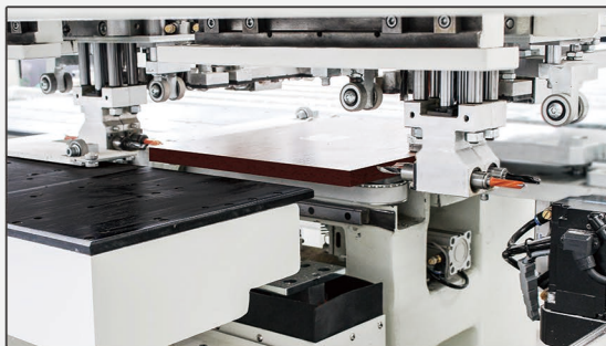
6-sided drilling completed in one cycle
