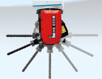
CNC machining center with 5 synchronizing interpolated axes
