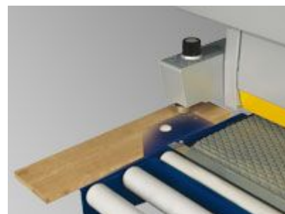
Automatic thickness measurement for high precision and productivity
