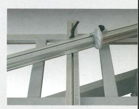
The double mitre system on the outrigger table with telescopic stop 2600 mm is standard for professional type machines.
