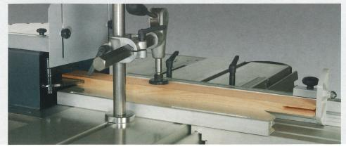
The Felder device for tilting the feeder away means the power feeder always remains on the machine and can be used at any moment without problems.
