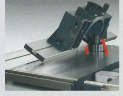
Professional Equipment: Spindle fence 240 for max. tooling diameter 230 mm, MULTI adjustment for spindle fence 240 enabling parallel running and quick setup
