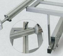
The scale on the crosscut fence is bevelled towards the operator, this is to assist you when setting the crosscut-stop position improving accuracy by preventing readout errors. The crosscut-stop position-indicator is perfectly integrated into the body of the crosscut-stop.
