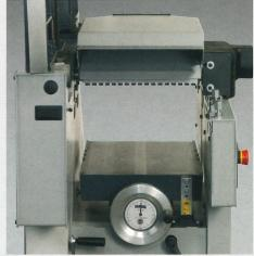
The horizontal mortiser is mounted on the planer side. The mortiser carriage may have a dowelling device or not, depending on what you require.
