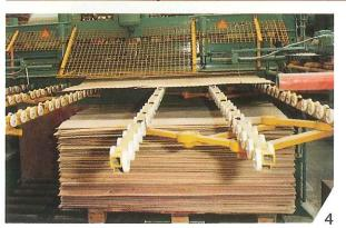
**4 Veneer stacking system**Designed to stack different sizes of lay-ons individually.
