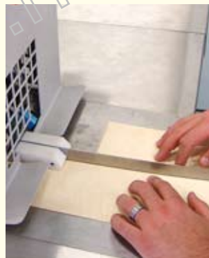
Automatic veneer infeed after manual alignment
