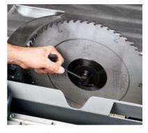
Simple, safe & quick – "Quick-lock" saw blade clamping Quick and easy blade change with only one tool, thanks to the "Quick-lock" system.
