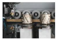
Two counter rotating, separately controllable spiral jointing cutters
