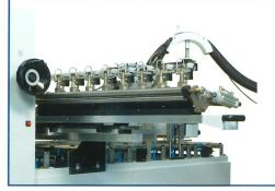
The adhesive application unit of Optimat FKP 100/DH can be extended at the side for maintenance and set-up work.
