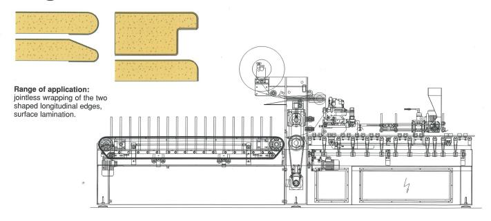
Due to the modular machine concept of the Optimat FKP 100 production series, the system can also be exclusively used for surface lamination (FKF). For this purpose, the wrapping zone is replaced with a chain conveyor. The two versions can of course be equipped for the processing of hot-melt-type adhesives (version DH) as well as for the processing of foils with adhesive coating at the rear (version VH).
