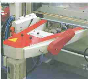
Belt sanding unit for profiled edges "S-7"
