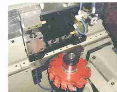
Pneumatic top pressure system on profiling unit
