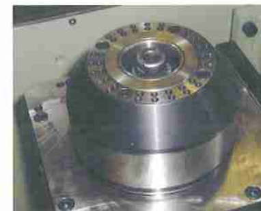
HSK 63 quick disconnect system on profiling unit
