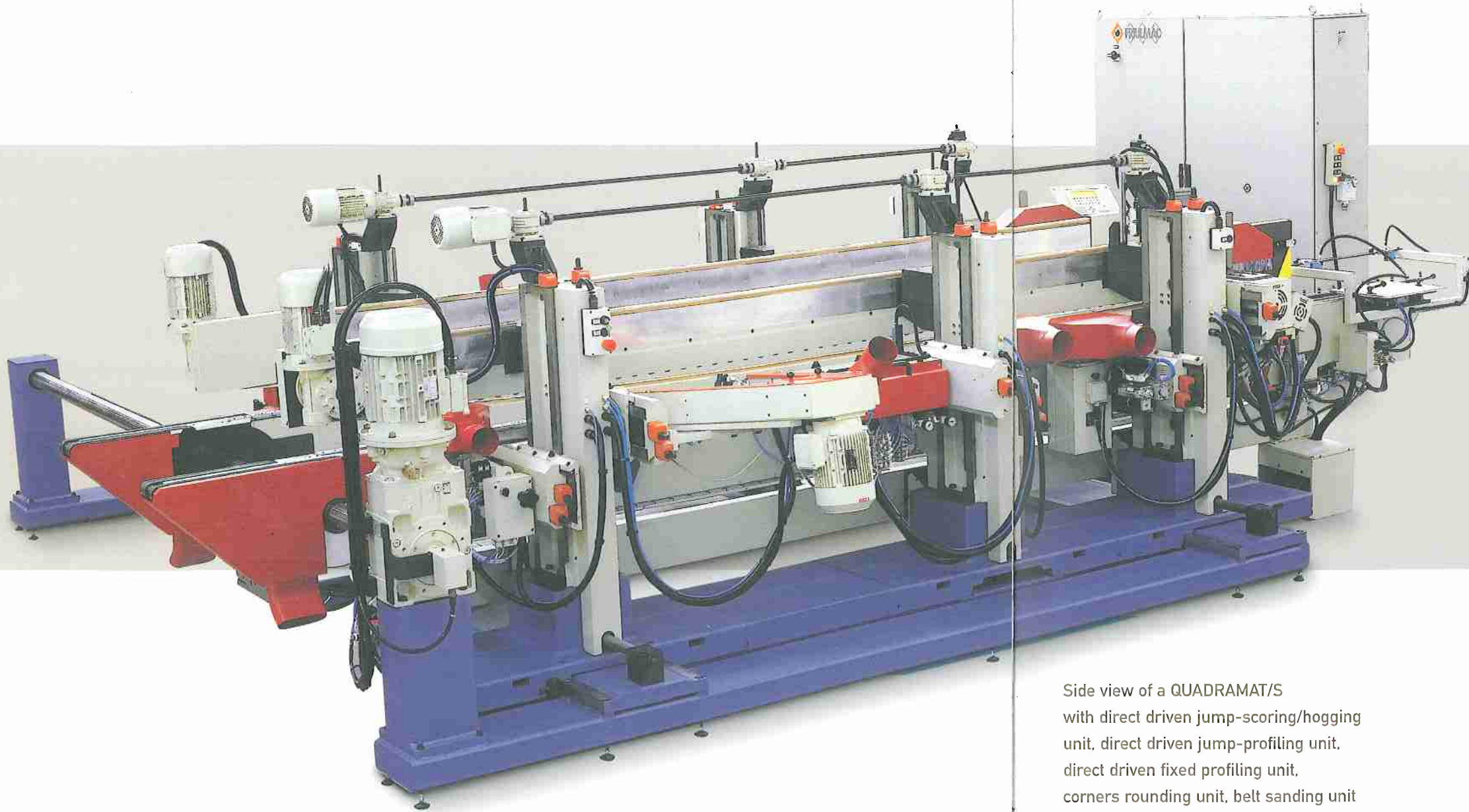
Side view of a QUADRAMAT/S with jump-profiling unit, direct driven fixed profiling unit, belt sanding unit for flat edges and disc sanding unit
