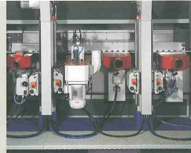
Side view of a QUADRAMAT/S with jump-profiling unit, direct driven fixed profiling unit, belt sanding unit for flat edges and disc sanding unit
