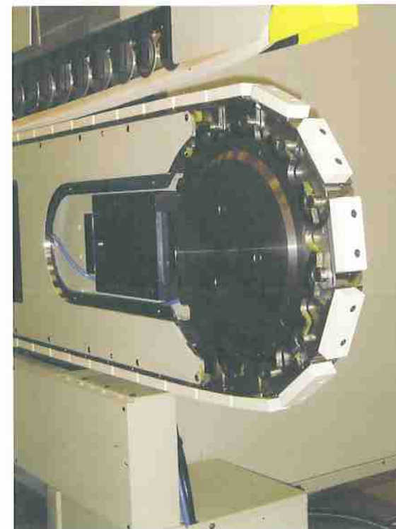
Detail view of the sliding feed chain system narrow type for short pieces
