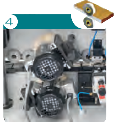
4 BUFFING UNIT with 2 motors 0.37 kw with cloth discs dia. 150 mm.
