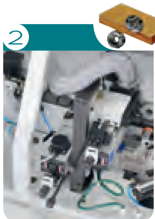
2 FINE-TRIMMING UNIT with 2 tilting 0° - 35° HF motors and micrometric adjustment with digital numerical read-out. No. 2 Cutters radius 2 mm.
