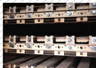
Jet box in saw tooth tread design
