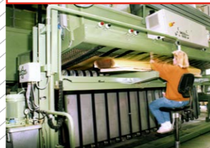
Half-automatic infeed system for sliced veneer
