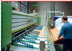
Vacuum outfeed system of slicer machine
