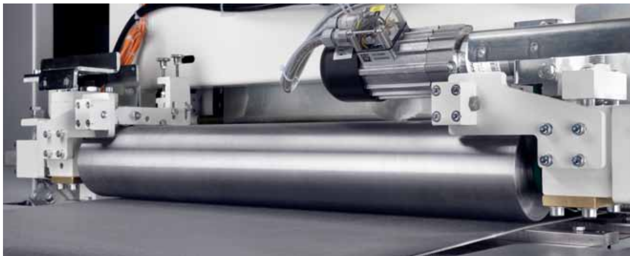
Control for excessive work piece thickness
