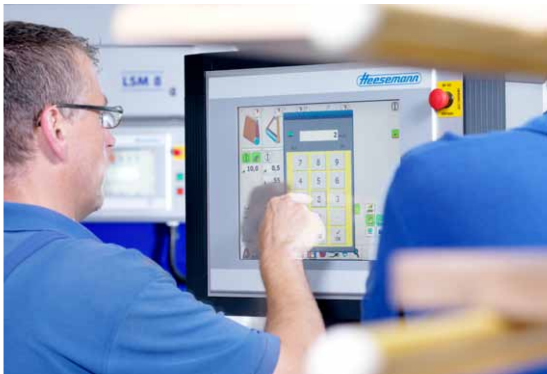
The industrial PC of the KSA 8 has a screen size of 15".
