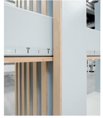
Pressing surfaces with tolerance compensation: The pressing lamellas work as a unit; they are placed on rubbers and suspended. Pressure is very evenly distributed due to the fact that the pressing lamellas simultaneously impinge on the carcass. Tolerances in the carcass are better absorbed.
