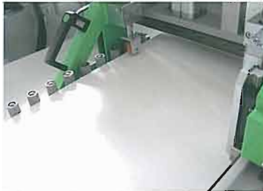
Side pusher with automatic pressing unit.
