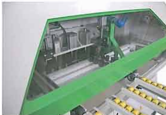
Possibility of panel unloading either on the back roller table or on the front with return of the processed panel to the operator.
