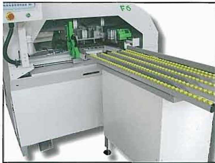
F6 model with fixed roller table for panels of big dimensions.
