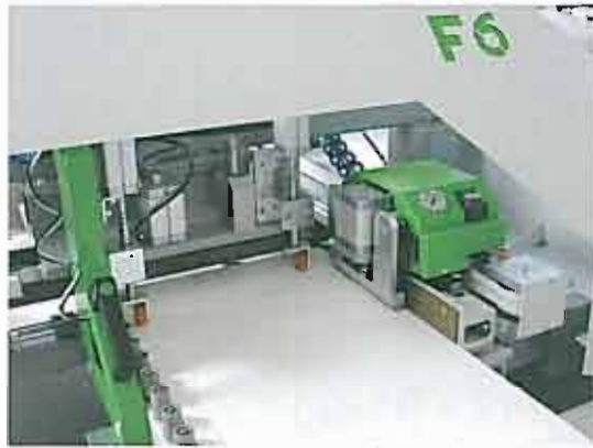
System of panel seizing and feeding by automatic clamps.
