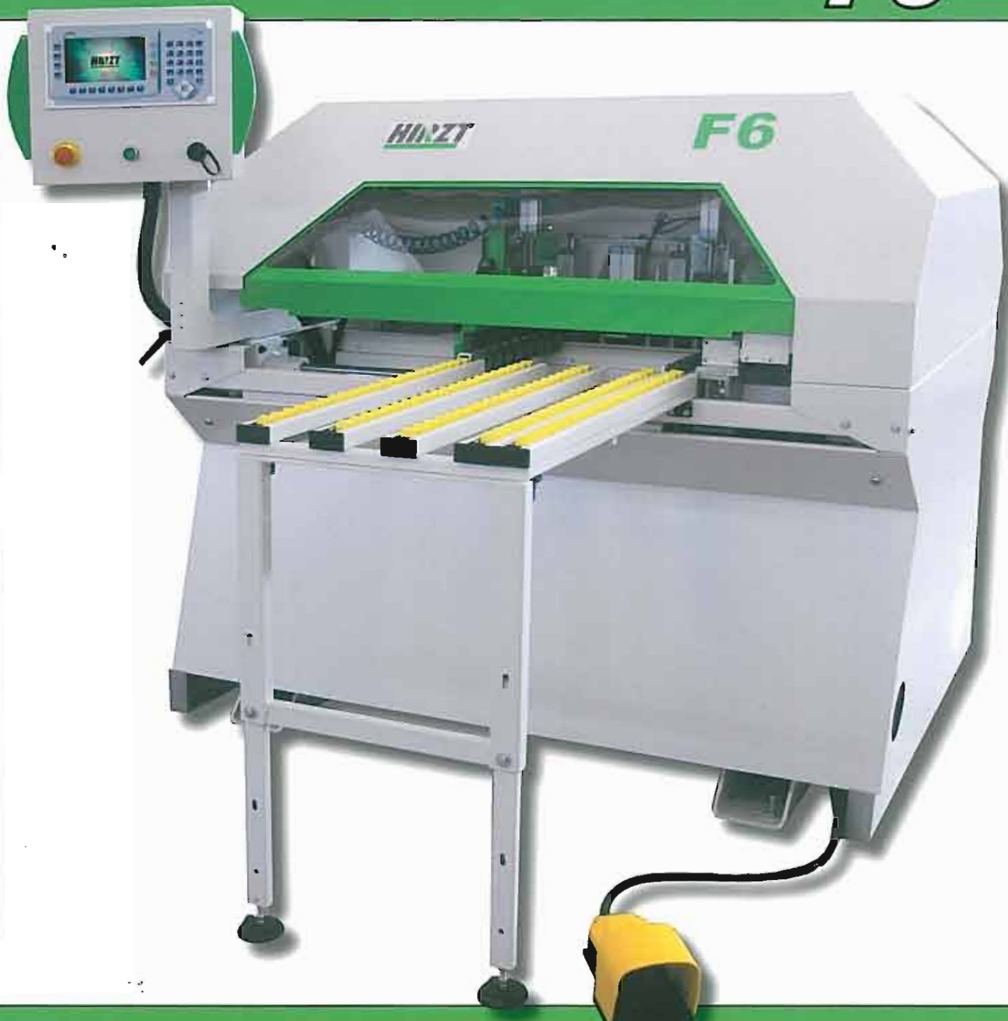
F6 model with folding roller table and sliding door protection.
