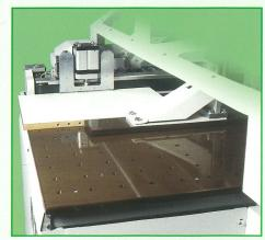
For processing in series it is used the back unloading system that allows a one after the other panel unloading. It is possible to program processing sequences of big and small lots by reducing time because in the process are eliminated positioning and loading times.
