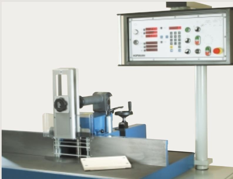
**Commitment to quality and flexibility.** Operating panel for top operating console. The quality is in the detail: Optional safety rulers with milling board and Centrex safety guard.
