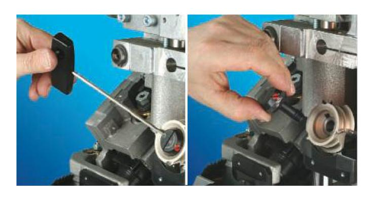
PRO-LOCK screw-in spanner for easy and quick tool change
