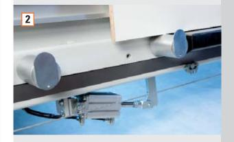
Automatically lift down of the roller during plunge-in of the saw blade. For high accuracy of the cutting dimensions [figure 2].
