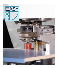
easyEdge edge banding unit: The world's smallest edge banding machine – affordable, simple, efficient. The universal solution for edging small workpiece quantities with veneer edges, ABS edges, PP edges, melamine edges and thin PVC edges. In conjunction with a manual snipping unit, it is even possible to perform 360° butt joint edge banding in craftsmanship quality.
