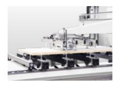
**Alignment against stops:** Articulated suction grippers permit precise positioning of workpieces against the stops on the machine table.
