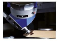
Routing of a dovetail joint for upright / transom constructions
