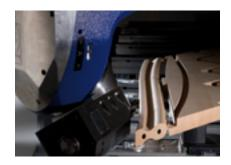
Holes for paling at narrow angles
