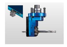
Lock case trimming unit with 2 toolholders: For trimming operation such as lock cases and lock face plates in doors, with integrated air jet for optimum chip discharge. The unit has a two-sided spindle outlet for two tools with a maximum useful length of 135 mm / 35 mm.
