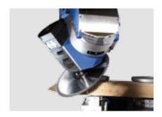
**Five-axis trimming spindle:** Compact DRIVE5C/+ five-axis spindle with 10 kW output (optionally 12 or 15 kW) and a controlled spindle speed of 0 to 24,000 rpm for high torque even at low speeds.
