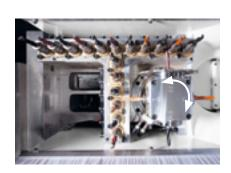
**Drilling head V17/H4:** HIGH-SPEED drilling head up to 7500 rpm with 17 vertical spindles, grooving saw and 4 horizontal spindles with 0/90° swivel facility. Fast drilling including grooving in the X/Y direction.
