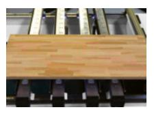
**Laser projection** of the clamps and the workpiece contour for optimum utilization and simple positioning of raw parts which cannot be aligned at the stops.
