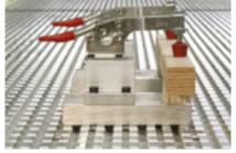
Fixture using non-standard clamps: The aluminium grid table with dovetail guides guarantees precise, positive fitting clamping element fixture.
