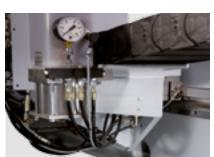
Covered linear guides: Covered linear guides with closed guide carriage and integrated central lubrication of all axes. Closed energy chains to protect against damage to cables and hoses.
