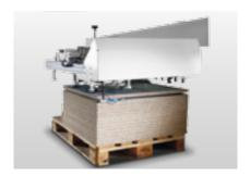
**Gripper technology with a system:** Integrated sensor functionality prevents errors as a result of adhering parts, while monitoring that workpieces are correctly picked up.
