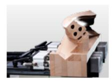
**Clamping device:** Uprights and staves can be securely clamped in no time using this clamping device.
