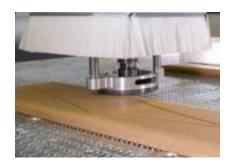
sensoFlex tracing system: Perfect workpiece quality – the traced spindle compensates for unevenness and unwanted tolerances. Tracing facility for different tools ensures complete flexibility
