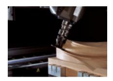
Routing of a stair hand rail
