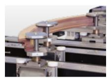
**3-step clamp:** Highly rigid 3-step clamps with extreme clamping height for precise complete processing of window and front door components without subsequent outside moulding and profiling.
