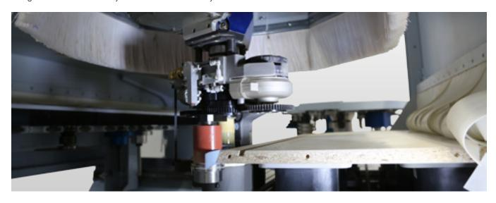
easyEdge and DRIVE5C+: The perfect combination of edge gluing and high-performance 5-axis processing. The DRIVE5C+ spindle engages the easyEdge unit directly from the pickup station in the lateral linear changer, the edging material is fed in – done.
