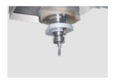
Minimum quantity lubrication: Machining of aluminium with minimum quantity lubrication through the unit or by means of an external spray pipe at the spindle for maximum care of tools.
