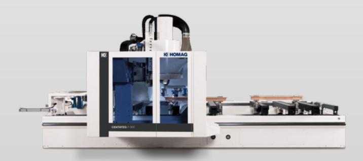
**CENTATEQ P-300:** Processing centre with 3-step clamping system for window manufacturing
