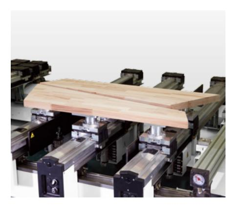
**movePart:** The clamps move apart automatically in the program sequence after separation for complete processing.
