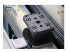
**Suction cups** are displayed using a laser beam (cross hairs). The workpiece contour can be "travelled" as a positioning aid for freeform part.
