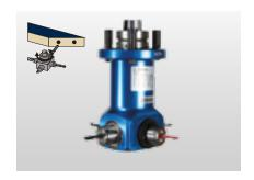
2+2-spindle drilling/trimming unit: The 4-sided spindle outlet makes available four different drilling and trimming tools without tool change. Continuous shaft for greater rigidity and processing without change of direction when using clockwise and counterclockwise rotating tools, e.g. when trimming out recesses for door hinges.
