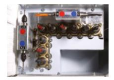
**Drilling head V9/H4:** HIGH-SPEED drilling head up to 7500 rpm with 9 vertical spindles and 2 horizontal spindles in the X direction and 2 in the Y direction
