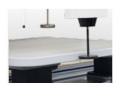
**Measurement probe:** Tracing system to determine the actual X, Y and Z axis measurement of relevance for processing with automatic correction offset in the processing program.
