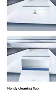
Fast and convenient: The area under the saw carriage is easily accessible via flaps, allowing easy removal or vacuuming of cutting waste.
