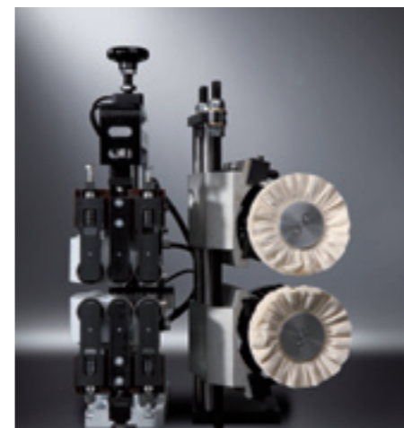
Finish processing FA11 the scraping device glue joint and the buffing device put the "finishing touch" to the workpiece
