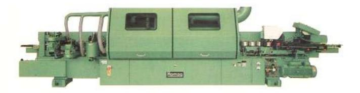
Edge banding machines single-sided KL 30 double-sided KL 40 For gluing and processing of thin and thick edge strips according to the hot cold method (hot-meth) or cold-glue activation method (KA) with PVAC-glue. On request noise protecting cover and centralized auction.
