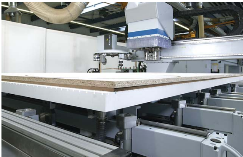
The raw panels (up to 2,800/2,100 mm) are positioned on an MDF vacuum spoil board.
