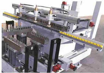
Horizontal drilling support with 21 spindle-drilling head, pneumatic workpiece clamps, panel stop and height adjustment according to panel thickness
