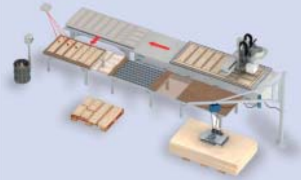
Handling tables for nesting with Mr Beam laser system for part identification
