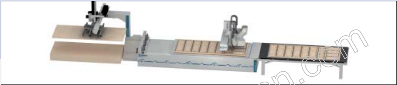
Used in conjunction with the TBA feeder, the pushing device with integrated extraction, air cushion function and an outfeed conveyor table,
