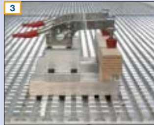
3 Aluminium matrix table with dovetail profiles for positive locking, flexible fixture of clamps
