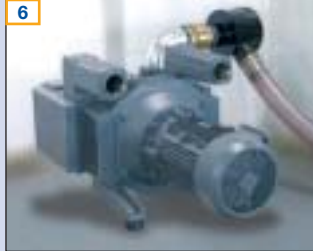
6 Vacuum pump with 500 m 3 /h output; 4 inch pipework in the basic machine for transmission of large vacuum flows
