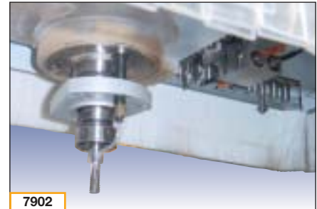
Tool holder with cleaning air jet for improved extraction output during nesting
