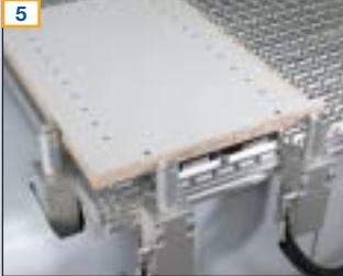
5 Stop dogs for simple, secure positioning of workpieces, also for alternating processing
