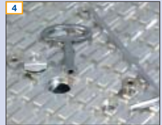
4 1" vacuum connections with quick-action opening using a switch cabinet key, vacuum openings with fine thread for fixture of clamps
