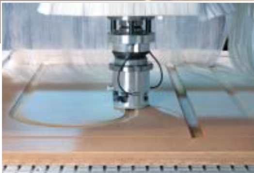
Vertically traced trimming unit for highly precise processing of, for instance, furniture fronts
