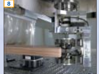
8 Interpolating C axis 360°: To allow the units to be rotated at any optional angle, including transmission of compressed air into the units (e. g. for traced units)
