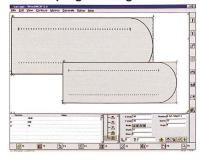
wood**WOP** is configured for variable part programming. This allows coordinates and technological parameters to be entered not only using values but also variables and formulas, so permitting the generation of variant programs. The side of a cabinet, for instance, is generated only once.
