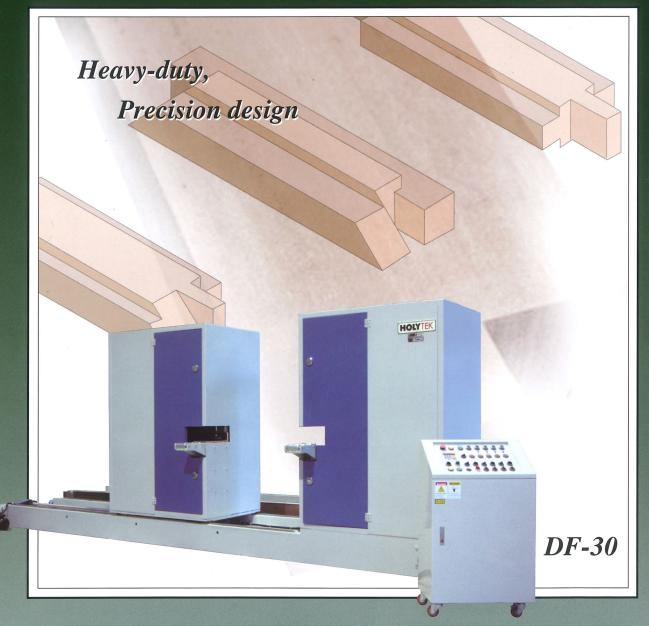
The Double End Door Frame Machine from HOLYTEK, available now. Max. working length up to 2.5m / 3.0m, width up to 200mm. Heavy rigid design with linear rail, ball screw width setting, electronic digital readout and full hydraulic control ensure stable and vibration-free performance. All-enclosure safety guard to match CE standards.
