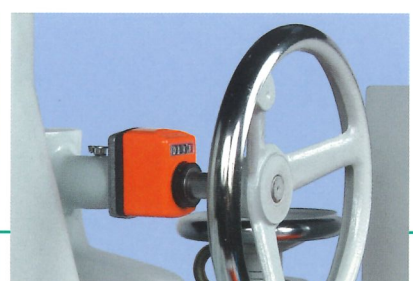
MECHANICAL DIGITAL READOUT OF ELEVATION WHEEL FOR PRESSURE ROLLS
