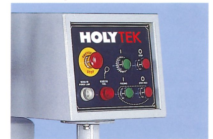
CENTRALIZED CONTROL PANEL
