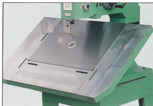
HR5 Overarm Router Table can be tilted to 45° and extended up to 1010×660mm (on request)
