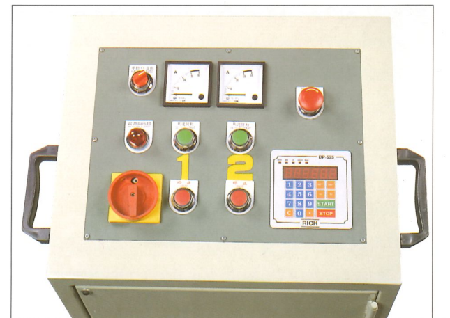
CENTRALIZED INDIVIDUAL CONTROL PANEL WITH DIGITAL READOUT FOR SETTING SIZE, AMPERE GAUGE PREVENTS OVERLOAD OF SANDING JOBS
