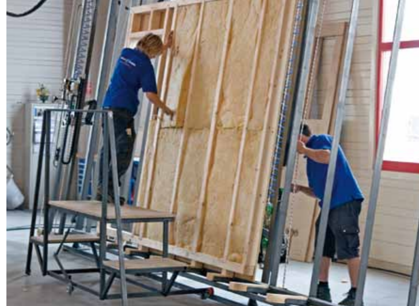
Montagepult MP Speed Wall System MP
