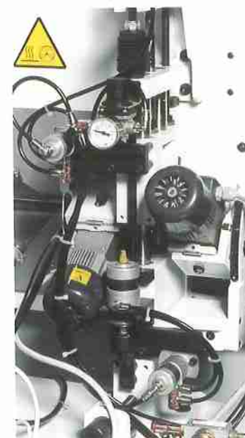
Staining unit Färberaggregat
