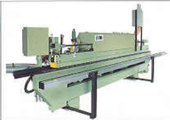
The side support bar is designed so as to reduce the lateral dimensions of the machine.
