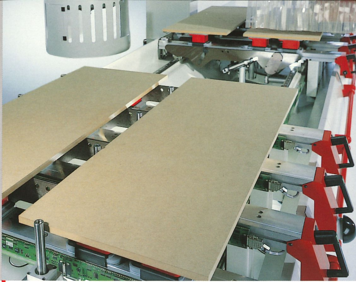
Panel loading using a second row of Y stops
