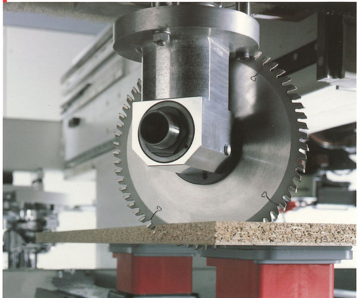
Main spindle with C-axis and adapter unit saw
