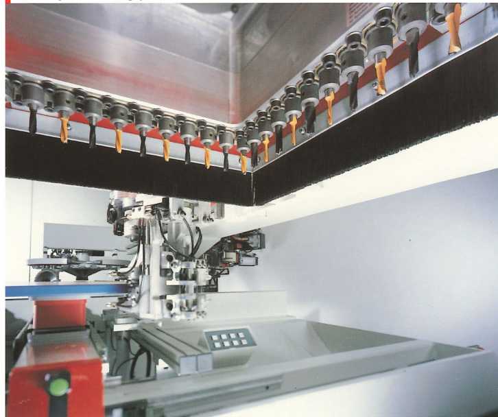
Boring head max. 21 drills, incl. 1 open docking place for attachment units
