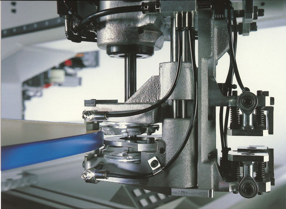
Combi adapter unit: flush-milling and flat scraper
