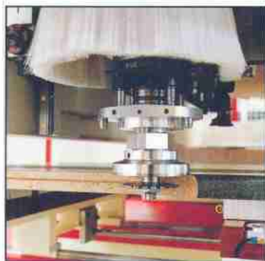
Adapter unit, horizontal grooving, tracing, CNC-controlled, 360 degrees, max. 5 mm tracing tolerance, rotation max. 9000 rpm.
