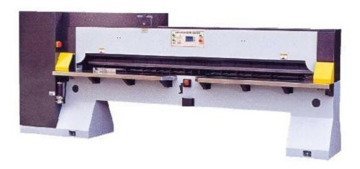
**Guillotines** - Heavy Duty Veneer **guillotine** with hydraulic pressure and operation complete with power rear feed unit, millimetre counter, knife and fittings. Fitted with Siemens input controller.
