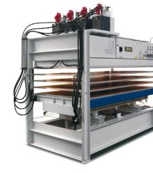
Alternatively heating by: - Heating unit elektric - central heating Water heating
