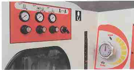
▲ Pneumatic pressure and easy Feeding speed control Three independent pneumatic controls for the setting of feed rollers. In feed and out feed rollers can be set with individual pressure. The EZ controls are positioned for convenient use.
