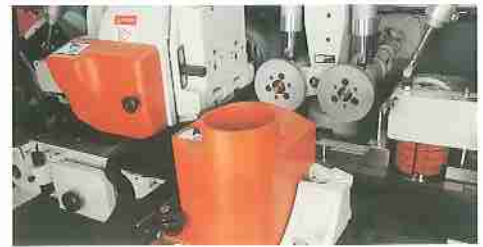
▲ Width vertical spindle cutter The 3th left vertical spindle is width cutter for setting the work-piece side to achieve perfect profile or straightness.
